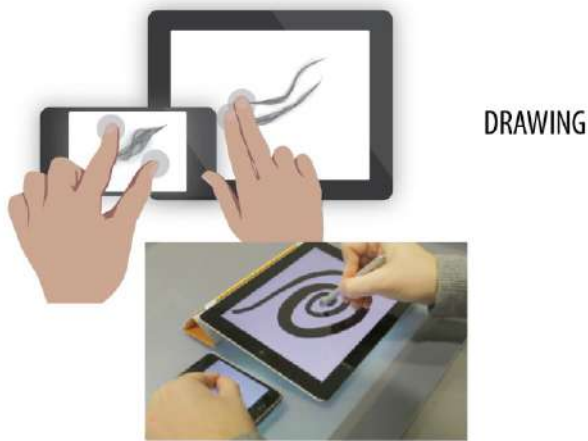
Fig. 7: Concept (top) and realization (bottom) of drawing on the phone and control on the tablet.
