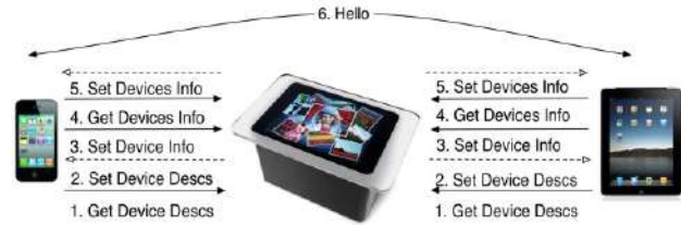
Figure 4: System structure and communication diagram between devices and Microsoft Surface.
